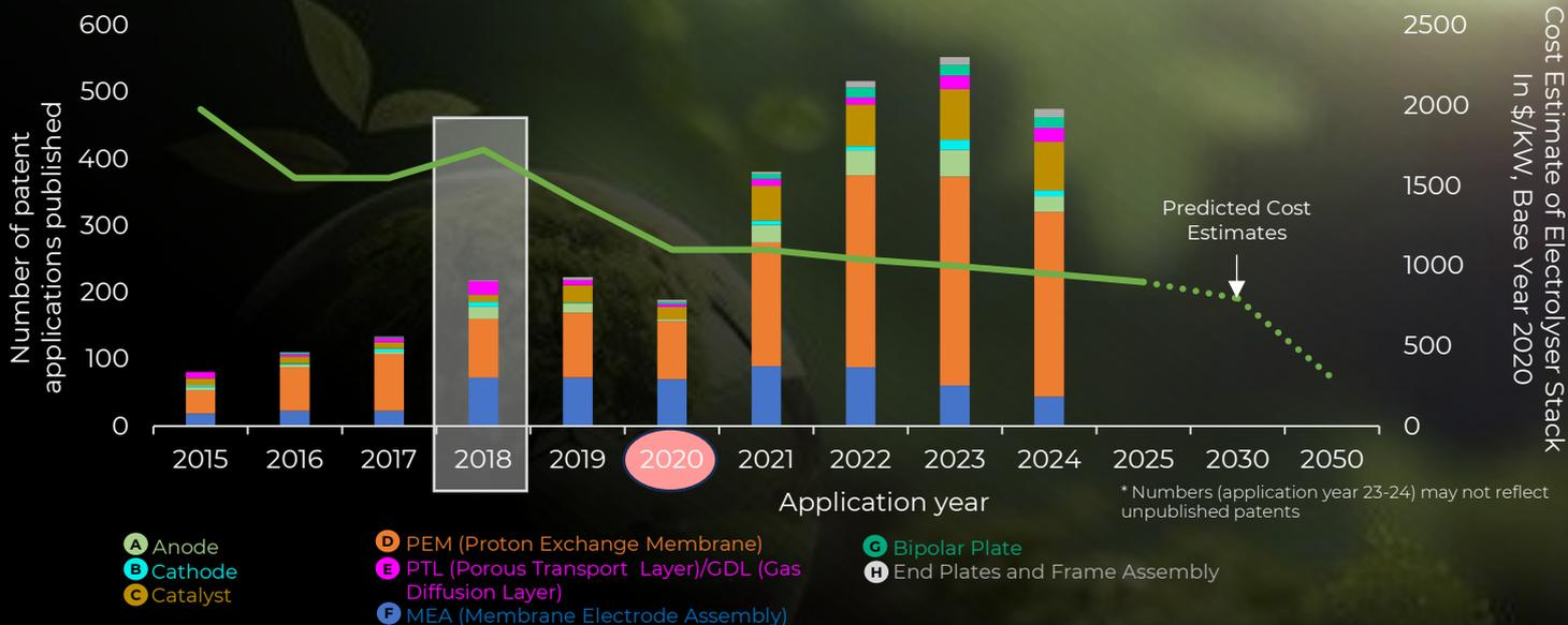
As illustrated in the graph, advancements in key stack components such as low loading of Iridium for anode, and alternate materials for catalyst and membranes are, accelerating. However, these innovations typically take 3 to 4 years to translate into cost reductions, reflecting the time needed for validation, scale-up, and integration into production.
